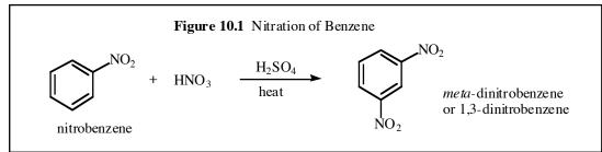
This reaction is an example of an electrophilic aromatic substitution. The nitro group is a strong electron withdrawing group and directs the incoming substituent
