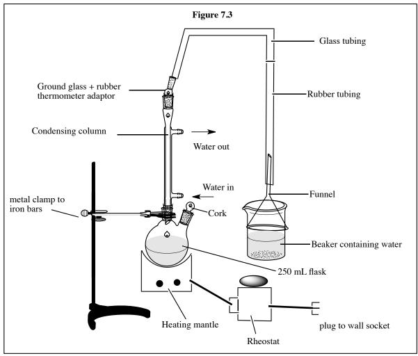
Attach the distilling column and glass absorption trap as shown in Figure 7.3. Add 2-3 boiling chips and heat the flask to a gentle reflux using a setting of about 60 on the rheostat. Again, the exact setting depends on the size of the heating mantle, etc. Do not heat too quickly as the reaction can get out of control and HBr gas can escape. If you do see HBr gas escaping immediately lower the heating mantle from the flask and call for assistance from your instructor or teaching assistant.
